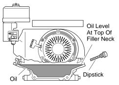
Figure 7 - Checking Oil Level (Model RGH5500A Shown)
